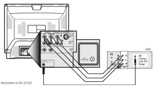
**To Connect:** Plug one end of the AV Compu Link cable into the AV Compu Link input on your VCR or other Compu Link device. Plug the other end of the AV Compu Link cable into the AV Compu Link input at the rear of the television.
